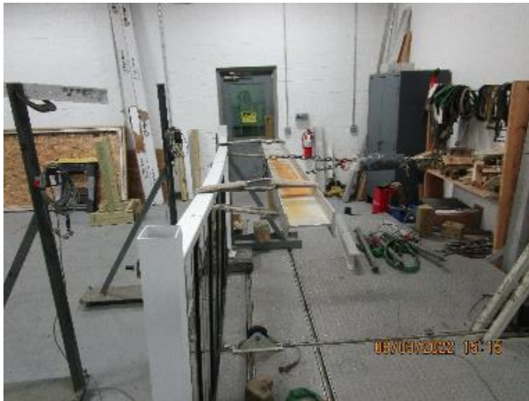
Photo No. 3 Horizontal Uniform Load on Top Rail
