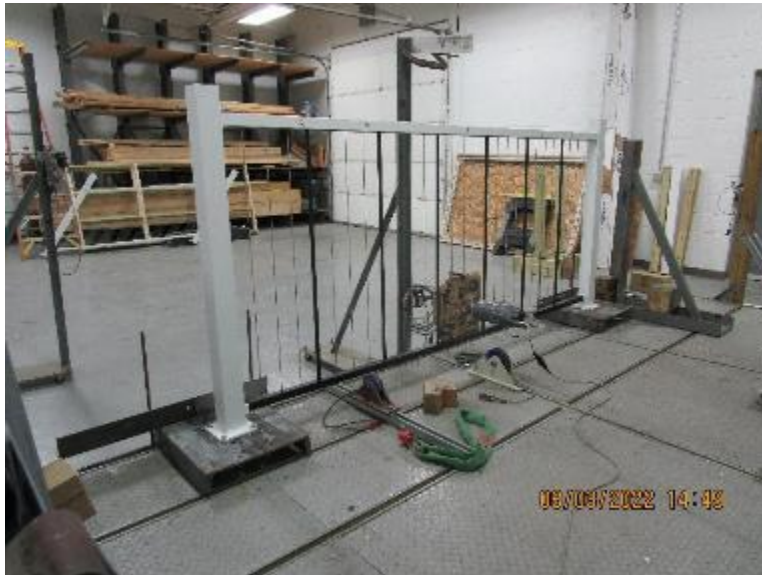
Photo No. 2 In-Fill Load Test at Bottom of Three Cables
