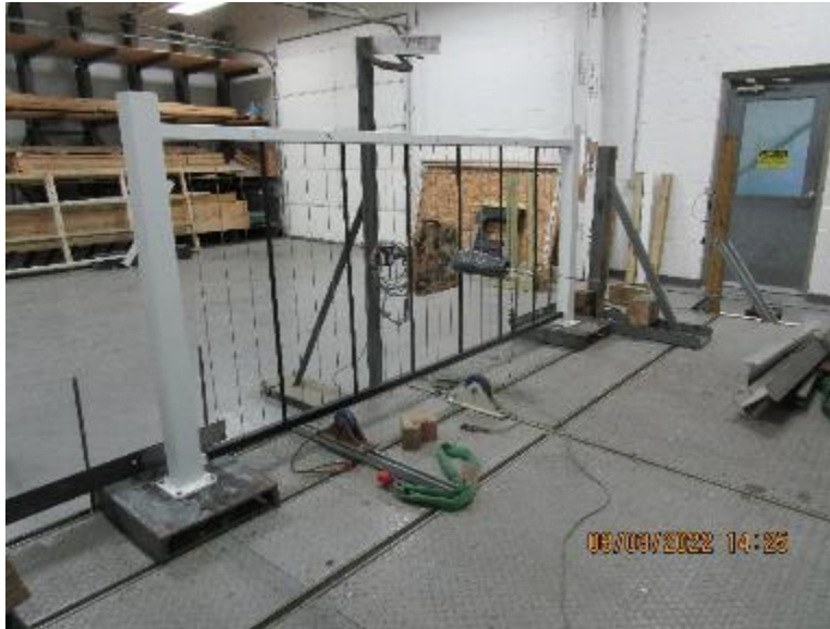
Photo No. 1 In-Fill Load Test at Center of Three Cables
